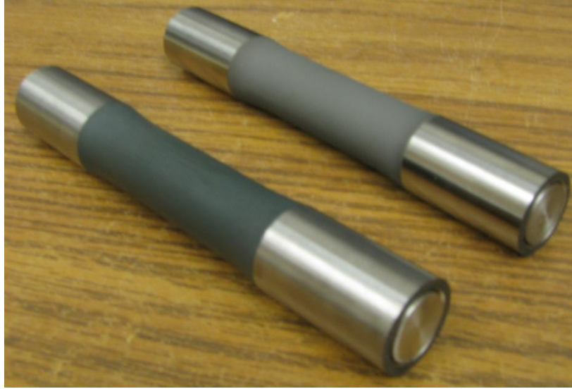
Figure 3.10: Uncoated (Left) and Coated (Right) Specimen After Modifications
