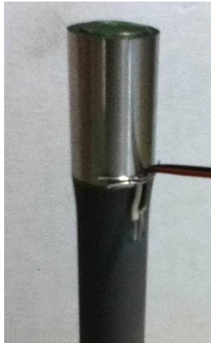
Figure 3.15: Thermocouple Attachment to Specimen
