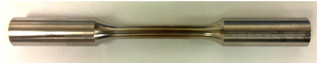
Figure 3.2: Solid Round Bar Test Specimen Normally Used at Georgia Tech
