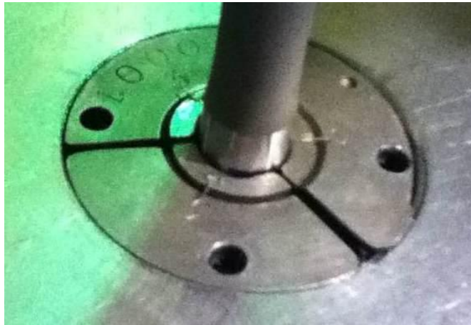
Figure 3.13: Specimen Gripped by Collet with Adapters
